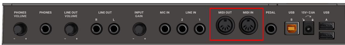
The MIDI sockets on the rear panel of MASCHINE+
