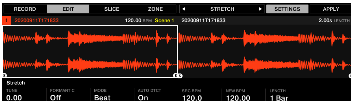
The Stretch controls at the bottom of the Edit page.
