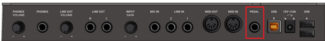
The PEDAL socket on the rear panel.
