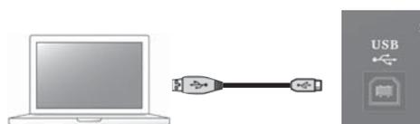
**You must install the USB driver when connecting the unit to your computer.**
