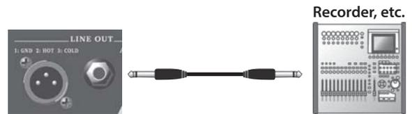
You can use this in conjunction with an external PA system, or to record your performance via direct line while monitoring the sound from the Nextone's speaker.
