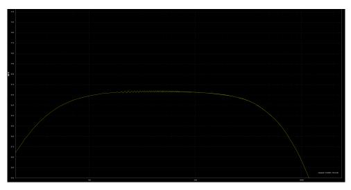
The ZIO can internally recreate the sound of a short cable run after the echo unit (as if it were sitting near or on top of the amplifier) and a variable length of cable in front of the unit, using the TONE switch. The combined effect gives a focus in the midrange without too much brightness or boomy bass.
