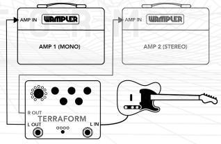
TERRAFORM will understand if you are running in mono - Make sure routing switch is set to **NORMAL**.
