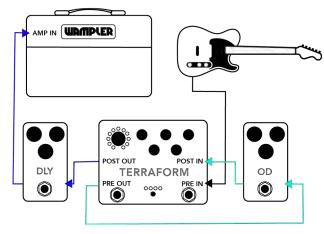
Make sure the routing switch is set to PRE/POST
