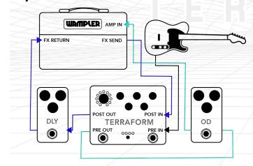
Make sure the routing switch is set to PRE/POST
