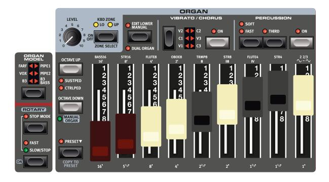
The Nord Electro 6 features five organ models, all digitally modeled: A B3 tonewheel organ with a dedicated B3 Bass mode, two transistor organs and two Pipe organ models, including a "principal pipe" section.
