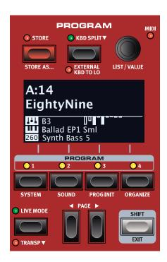
The **PROGRAM** section provides access to performance functions such as loading and storing programs, access to Live programs, keyboard split functionality and more. This is also where menus containing *System* and *Sound* settings are found. The menus and their settings are covered in a separate chapter, starting on page 26.
