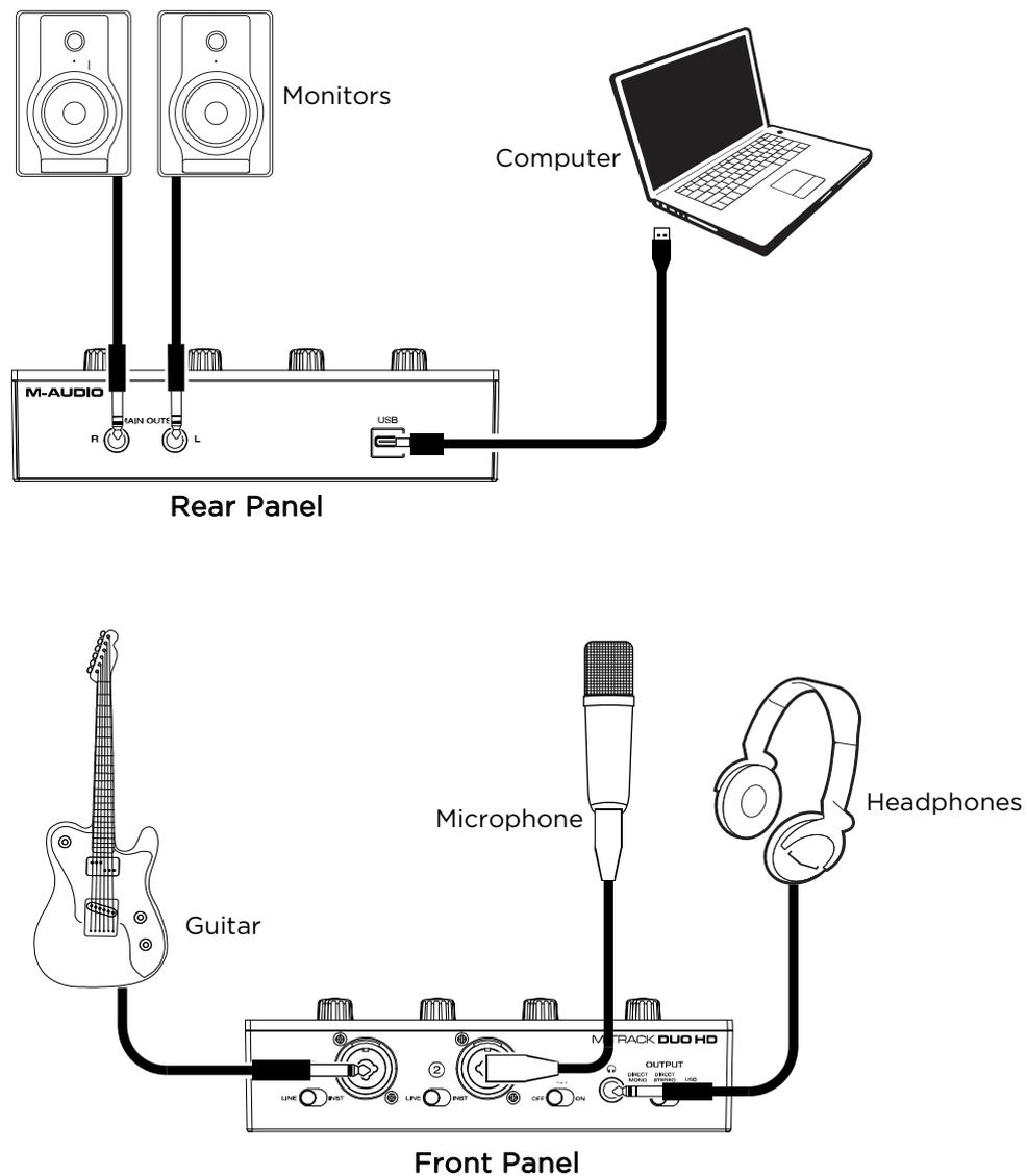
**Note:** Use the **+48V (Phantom Power) Switch** only if a microphone requires phantom power. Most dynamic microphones and ribbon microphones do not require phantom power, but most condenser microphones do. Consult your microphone's documentation to find out whether it needs phantom power.
