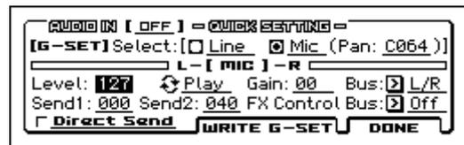
5. Use Bus (Bus Select) to specify the bus where the audio input will be sent. For example if you want the output of the device that’s connected to LINE IN to be input to insert effect 1, specify IFX1 as the Bus (Bus Select) setting when selecting the routing.
