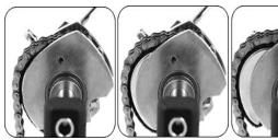
Torque position adjustments from eccentric (far left) to concentric (far right
