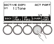
4. Press UPPER1, UPPER2, or LOWER to select the part for which you want to disable application of the effect. This causes the selected part indicator ("U1", "U2", "L") to disappear from the lower right of the display.
