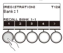
• If the last recalled bank number is selected, the area number will be displayed at the bottom of the LCD.
