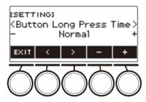
**5.** Rotate the dial or use – and + to change the button long-press time value.
