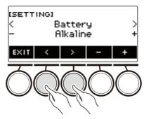
6. Rotate the dial or use – and + to select "Alkaline" (alkaline batteries) or "Ni-MH" (nickel-metal hydride batteries).
