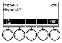
(6) Depress the heel end of the volume pedal and then press YES.
