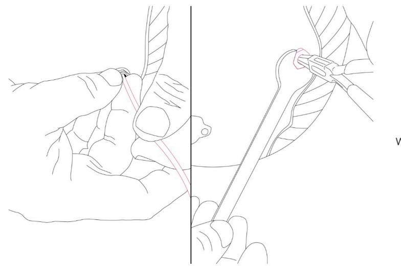
Place the washer and the nut on the outside of the jack and tighten. If needed, use pliers to hold the jack on the inside while tightening the nut on the outside. You may now remove the thread used to place the jack in the hole.
