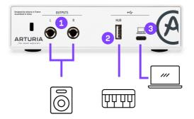
1 : TRS outputs to connect powered speakers or mixer/amplifiers
