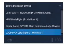
Once you change your system output to use the Loopback output, you will not be able to hear any computer audio until you a) record-enable a channel in your recording application, or b) switch the output back to "MAIN Left/Right" from the Speaker icon in the taskbar.
