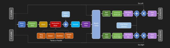
Each element in Artifakt has a discrete location in the signal path.
