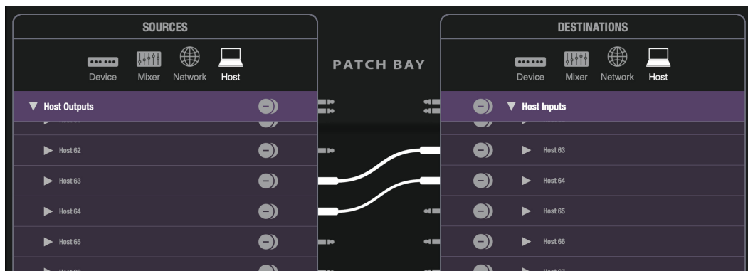
Figure 7-6: Creating loopback routing in the Patchbay. In this example, Host output channels 63-64 are being routed to Host input channels 63-64.
