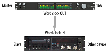
Figure 4-4: Slaving another digital audio device to the 16A via word clock. For the 16A clock source, choose Internal (or any source other than Word Clock , as daisy-chaining word clock is not recommended).
